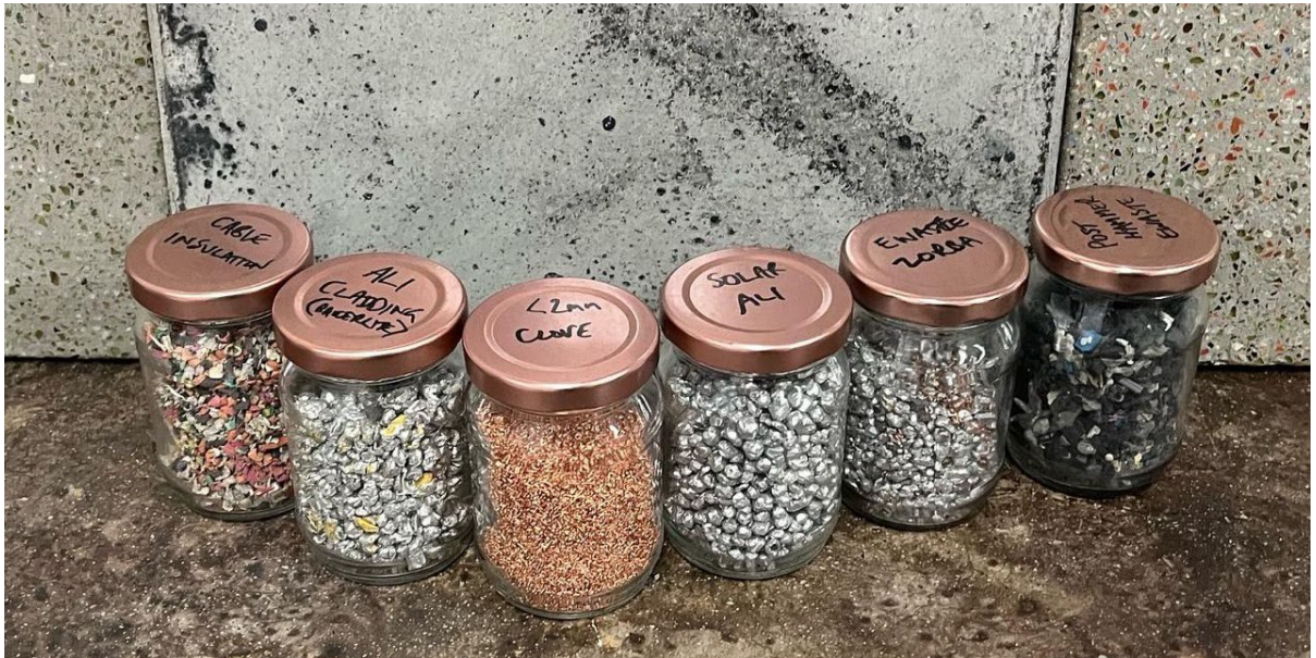
Figure 2-3: Cable insulation and other solar farm components after recycling
